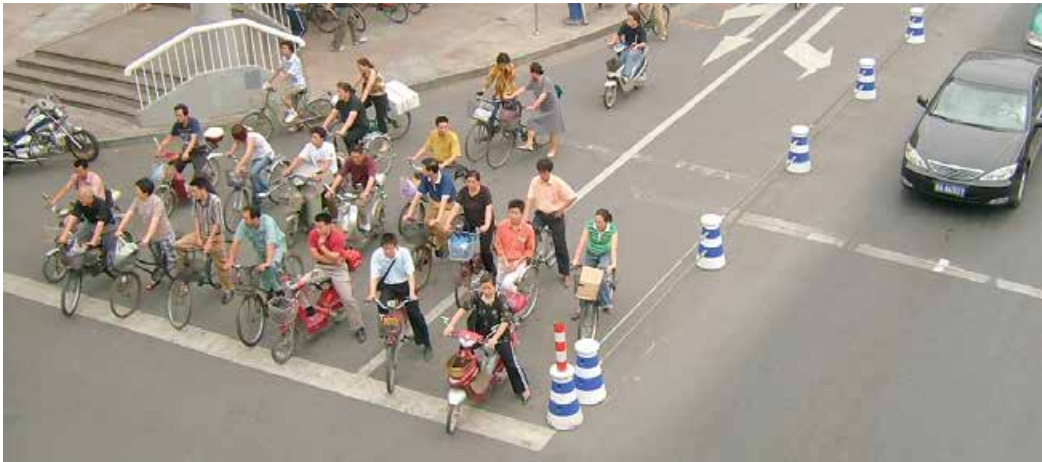
A high capacity cycle way has physical protection, turning lanes and an advanced stop line for cyclists in Hangzhou, China.
